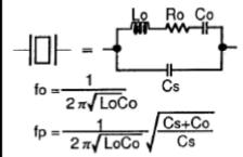
Fig. d: Crystal oscillator equivalent circuit
