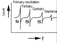
Fig. f: Overtone oscillation vibration level
