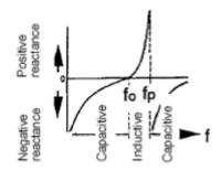
Fig. e: Reactance frequency characteristics of crystal oscillator
